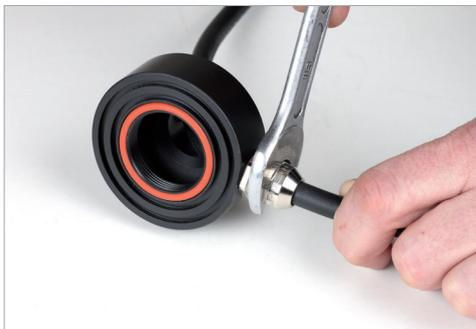
**1.5** Mount the cable and nipple into the Cable Entry Port body. Use a metric wrench (size 18) to gently rotate clockwise. Be careful not to damage the threads.
