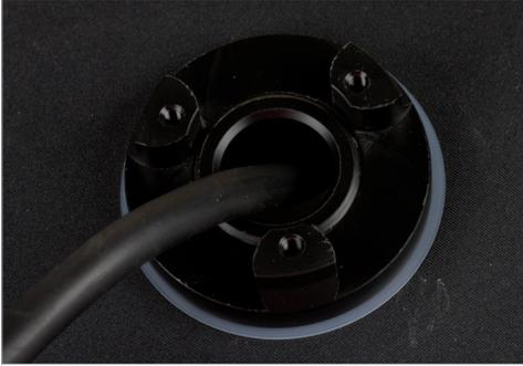
**2.3** Mount the Cable Entry Port into the drysuit and attach the body of the bottom lid. Position the Cable Entry Port in preferred direction and tighten it by force of hand. Tightening shall be made through rotation of the bottom lid body.
