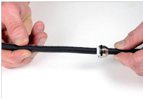
**1.4** Before next step it is important to measure the length of the cable for your specific need. When the nipple is mounted and fastened it will not be possible to adjust the cable in any direction without disassembly.
