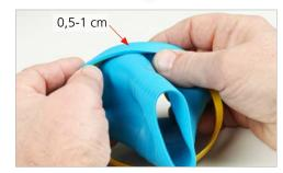
**1.1** Assemble the seal by inserting it through the **1.2** Push the seal and Spanner Ring assembly vellow Spanner Ring and bringing it back 0,5-1 cm over the yellow Spanner Ring. Note! The thin part of the yellow Spanner Ring should point outwards (when installing the assembly into the PU-Ring.)
