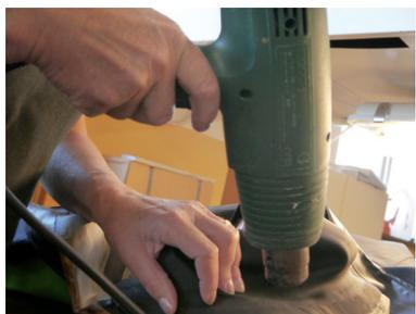
When the second coat of adhesive has dried, it is time to apply the rings to the drysuit. When you have fitted each ring to its actual position you will need to melt the glue by using the heat gun. You must be very careful when using the heat gun. If the fabric of the suit and/or component gets overheated you might damage it.
