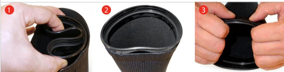
1. Folding the ring will ease the mounting process. 2. Raise the ring and place it with its flange approx. 8-10 mm from the edge of the drysuit arm. 3. Stretch the ring so that it connects to the suit 360°.
