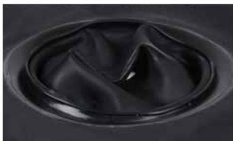
**1.5** Press with your fingers/with the Combi tool all around, until the Lock Ring and seal assembly has been forced into the groove in the Neck Ring. (Strive to get the same amount of excess part of seal around the entire assembly, see image 1.6.)
