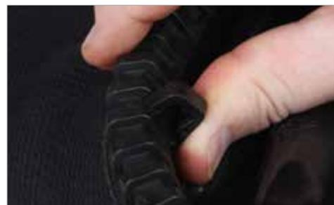
**2.3** Place the clip with the low tongue just below the all-around ridge of the ORUST Neck ring, as seen in the pictures. **NOTE:** The clip should be mounted from the inside of the ORUST Neck Ring.
