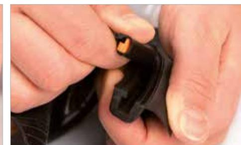
**3.3** The ORUST Neck Ring is designed for dynamic flexibility and will not demand tools for release of the Lock Ring and seal. You can easily release the Lock Ring by using your fingers. Grab the neck seal with one hand and bend (open) the ORUST Neck Ring with the other hand. Pull firmly until the seal and Lock Ring comes loose. **NOTE:** Be aware of the fact that sharp finger nails might damage the seal.
