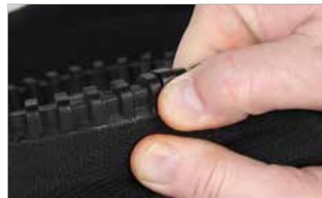
**3.1** Press with your thumb on the flat surface under the clip that you want to remove. Lift the bottom part of the clip with your other hand and fold the clip up- and backwards. If the clip is hard to remove by hand, you may use a tool to lift the clip up- and backwards. (For example the Combi tool, a screwdriver or other tool that has a flat and blunt edge.)
