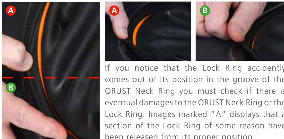
If you notice that the Lock Ring accidentally comes out of its position in the groove of the ORUST Neck Ring you must check if there is eventual damages to the ORUST Neck Ring or the Lock Ring. Images marked "A" displays that a section of the Lock Ring of some reason have been released from its proper position.
