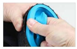
**3.2** SLÄGGÖ Flex Ring is designed for dynamic flexibility and will not demand tools for release of the seal and Spanner Ring assembly. Grab the seal and Spanner Ring assembly with one hand and bend it out of the PU-Ring with the other hand. Pull firmly until the seal and Spanner Ring comes loose. Note! Be aware of the fact that sharp finger nails might damage the seal.
