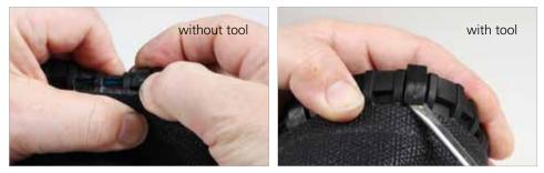
**3.1** Press with your thumb on the flat surface under the clip that you want to remove. Lift the bottom part of the clip with your other hand and fold the clip up- and backwards. If the clip is hard to remove by hand, you may use a tool to lift the clip up- and backwards. (For example a screw driver or other tool that has a flat and blunt edge.)
