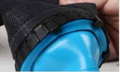
**2.2** Attach clip on every fourth compartment of the PU-Ring, totally six clips per PU-Ring. Inspect the assembly and pull the seal to check that all clips are locked in place.
