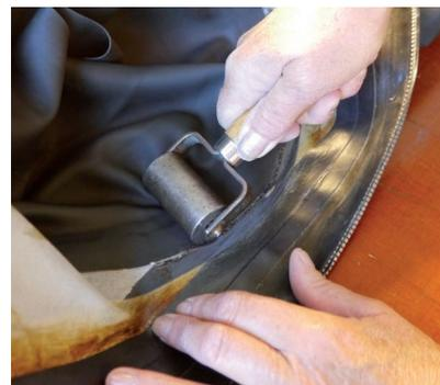
When the adhesive has melted and the ring is in place you need to squeeze away all air-pockets in order to get maximum grip between the components. Use a roller or similar tool to put equal force over the actual surface. Roll back and forth until you have covered the complete surface 360°. When this is done we recommend you to wait about 10 minutes before starting the next step.
