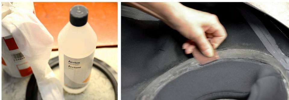
Ensure all surfaces are free from adhesive residues, debris and dirt. This is paramount for the glue to do the job. No matter the adhesive, tools or technique if not cleaned properly, the job will be sub-standard. Roughen the surface with fine emery cloth or sandpaper. Inhouse we use either a table grinder or emery cloth for roughing surfaces. The Quick Neck Ring shall be cleaned and de-greased by the use of acetone for maximum grip properties.
