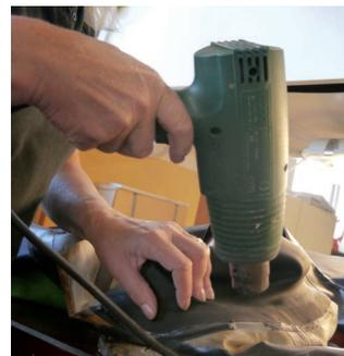
Heat both the Quick Neck Ring and the suit. Move the nozzle of the heat gun constantly to prevent the ring and suit from overheating. Work in areas of 5-10 cm at a time to keep the temperature of the glue at a smooth and constant melting point.
