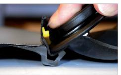
**2.4** Press up the Lock Ring from the groove.
