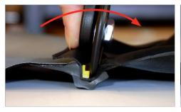
**2.3** When the tool has reached the bottom of the groove, it's time to use the tool to bend up the Lock Ring from the groove.
