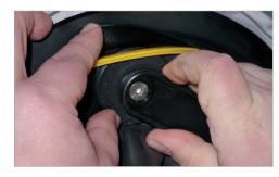
**2.5** When you have successfully released the Lock Ring you can use your fingers to pull the seal and Lock Ring out of its position.
