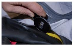
1.5 Push the Neck Tite Tool forward along the Lock Ring until all of it has been forced into the groove in the Neck Ring. (Strive to get the same amount of excess part of seal around the entire assembly, see image 1.6.)
