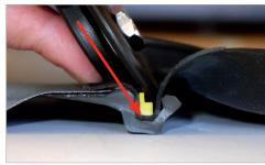
**2.2** Press the tool in the direction of the arrow and force the groove in the Neck Ring to "open up" and start releasing the Lock Ring.
