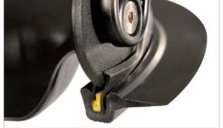
**1.3-1.4** Put the Neck Tite Tool in position as image displays. By applying force, press the Lock Ring down into the tapered groove of the Neck Ring so that the Lock Ring enters the groove and locks into position. **Use a flat surface when performing this operation.**
