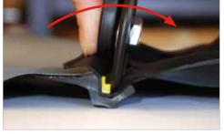
**2.3** When the tool has reached the bottom of the groove, it's time to use the tool to bend up the Lock Ring from the groove.
