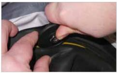
**2.1** Press the Neck Tite Tool towards the bottom of the groove in the Neck Ring. (See also cross section in image **2.2**.)
