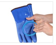
**2.1** Start by finding appropriate Spanner Ring. When pressing the Spanner Ring and glove into the Glove Ring they shall slide without use of excessive force. Use green Spanner Ring for thin fabrics, blue for medium fabrics and yellow for thick fabrics.
