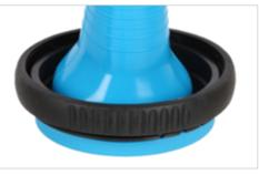
**1.7** Mount the seal onto the OBERON Ring as displayed in this image. Ensure that the flange of the seal is insterted into the groove of the OBERON Ring.
