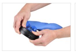
2.4 Press the glove with Spanner Ring evenly into the Glove Ring.2.5 Check for creases on the glove as creases may cause leakage.
